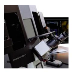
Installed 2018. Inverse widefield microscope equipped with a 4-Megapixel sCMOS camera for fast fluorescence and brightfield imaging. Sedat setup with filters for all conventional dyes from blue to deep red. 7-color solid state light source for fluorescence imaging with Köhler and critical illumination, respectively. White LED for brightfield, DIC optics. Motorized XY stage, hardware autofocus and environmental chamber for temperature and CO<sub>2</sub> control, onboard deconvolution.
