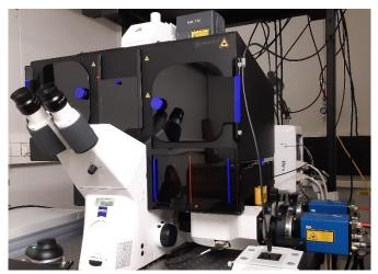
Installed 2022. Super-resolution microscope for lattice SIM, 3D SMLM (PALM, STORM), TIRF and laser widefield imaging. Dualcamera port with 2 sCMOS cameras for fast acquisitions. Apotome mode for thick specimen. Lasers to image dyes from blue to far red. Multi-positioning (Piezo-driven XY stage with Z-Piezo insert) and hardware autofocus. Environmental box for live imaging with temperature and CO<sub>2</sub> control (Last updated: May 2022)
