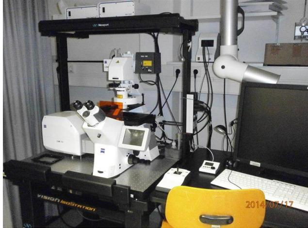
Installed: July 2014. Inverse point scanning confocal microscope with 2 PMT channels. Variable dichroic crystal configuration also allowing (slow) spectral imaging), transmitted light PMT and motorized stage. Widefield illumination: halogen (transmitted) and CoolLed pE-2 LED (reflected). ZEN 2012 acquisition software including "tiling & stitching" macro for larger overview imaging. Environmental control (stage-based) possible upon request.
