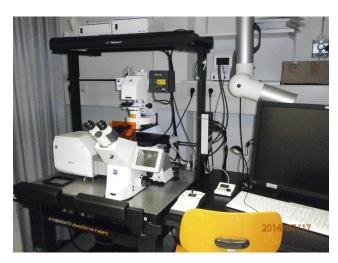
Installed: July 2014. Inverse point scanning confocal microscope with 2 PMT channels. Variable dichroic crystal configuration also allowing (slow) spectral imaging), transmitted light PMT and motorized stage. Widefield illumination: halogen (transmitted) and CoolLed pE-2 LED (reflected). ZEN 2012 acquisition software including "tiling & stitching" macro for larger overview imaging. Environmental control (stage-based) possible upon request.
