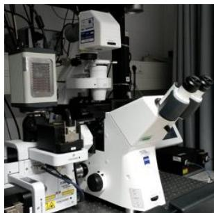
Installed 2012. Inverse spinning disk microscope unit for fast pseudo-confocal imaging, preferably for live applications at ambient temperature. Equipped with laser lines for blue, green, red and far red dyes. FRAP/photomanipulation with all laser lines possible. Fast sCMOS and high-sensitivity EM-CCD camera. Hardware autofocus, multi-positioning and stage-based environmental control, including a fast heater/cooler for temperature shift experiments.
