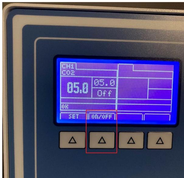
When finished with your session you need to shut off the CO<sub>2</sub> controller first at the front control and second at the back again. Do not forget to close the main valve at the flask.
