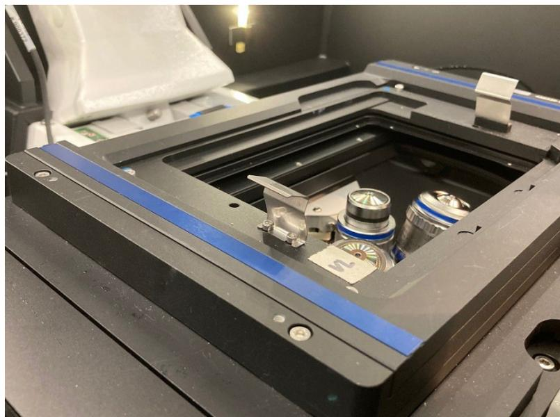
The insert for this Piezo controlled stage holder requires some assembly as it actually consist of two parts: one labeled Pecon and an additional insert. The additional insert allows you to adapt the chamber for your sample container. We can accommodate slides and Petri-dishes.
