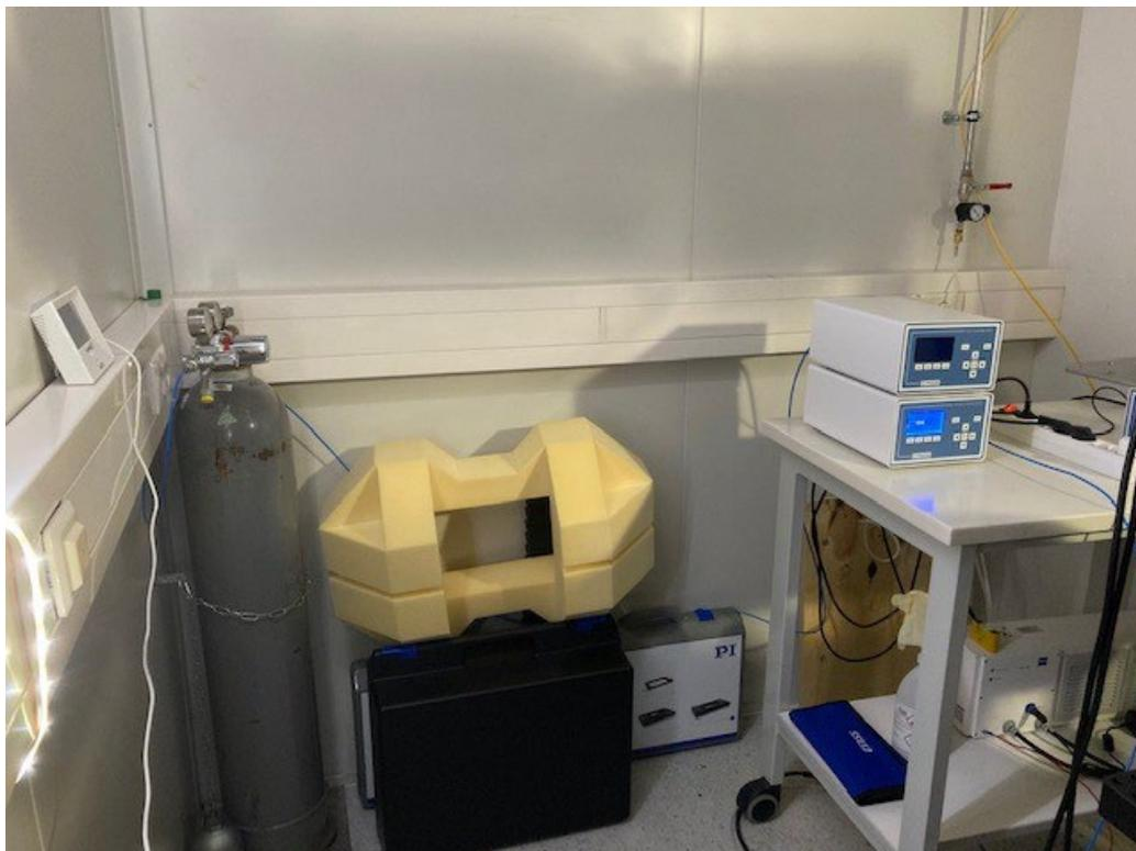
Remember: you need to open the flask at the main valve (bottom right image) **and more important at the end of a session CLOSE again** to use CO<sub>2</sub> at the microscope. Do not change the other valves on the manometer.
