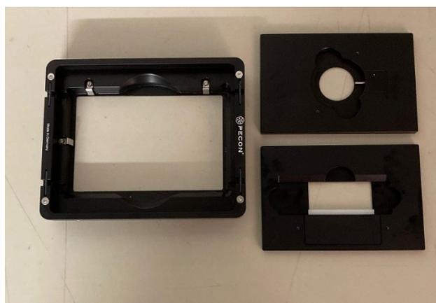
The final assembly for slide imaging is shown below. **Make sure to have the the objective in LOAD position when assembling the stage.** It is usually easier to put the smaller insert into the PECON frame before installing this on the Piezo controlled stage holder.
